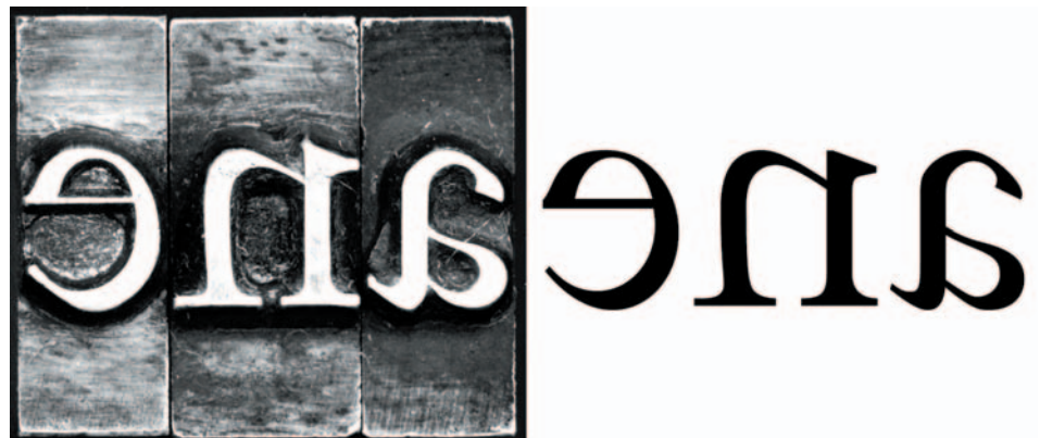
Types from Bembo metal (left); and Bembo digital (right).
